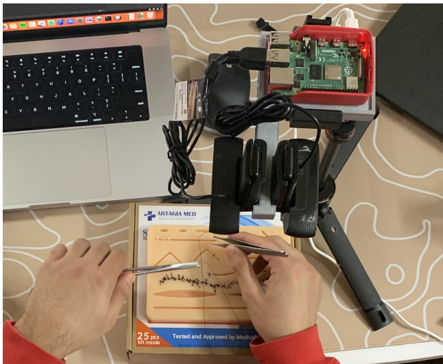
Fig. 4. The setup used for preliminary testing of the VR system. A trained medical student wore the VR headset and performed multiple sutures on a practice suturing pad guided exclusively by the images acquired by the cameras. The images were streamed through a private Wifi server. The focal length and camera angles were easily calibrated to achieve an optimal configuration.
