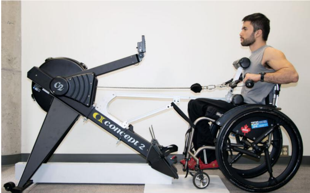
Figure 1. AROW adaptations to Concept 2. Adaptations for the Concept 2 include a support bar extending to the user's chest and a rigid attachment to the frame of the rower [2].
