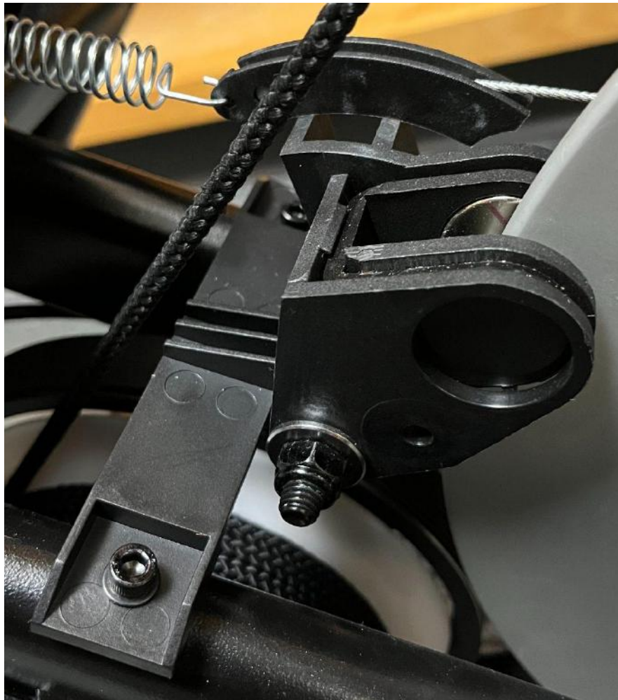
Figure 4. Previous Resistance Mechanism The magnet housing was originally screwed into the support portion of the two angled support bars that are within the plastic housing of the rower. The housing is one large piece of plastic that rotates about the central bolt shown above. The new resistance dial mechanism keeps this entire structure intact.
