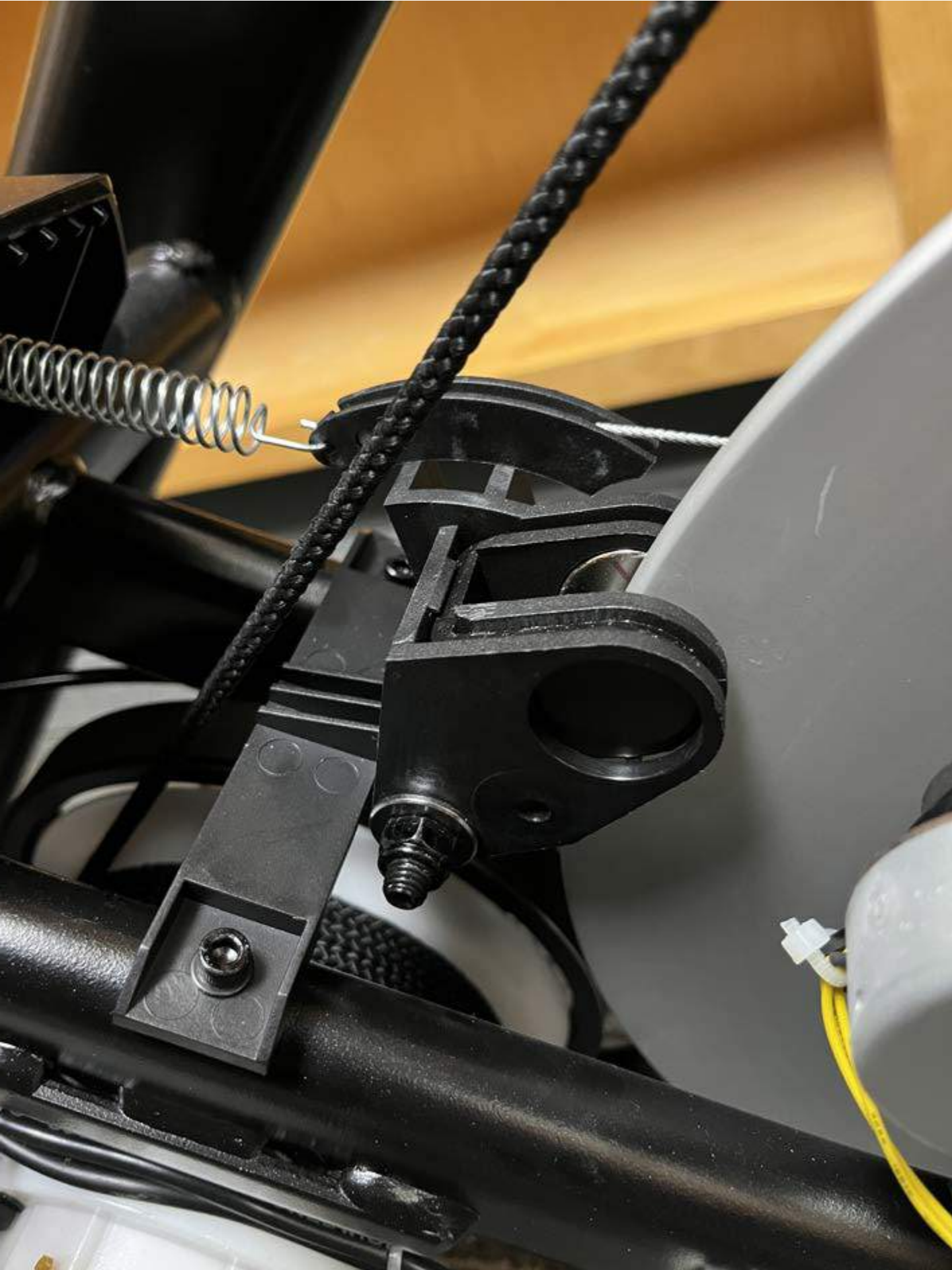
The above image shows the magnet housing and how it screws in to the two supports on the internal rotor.
