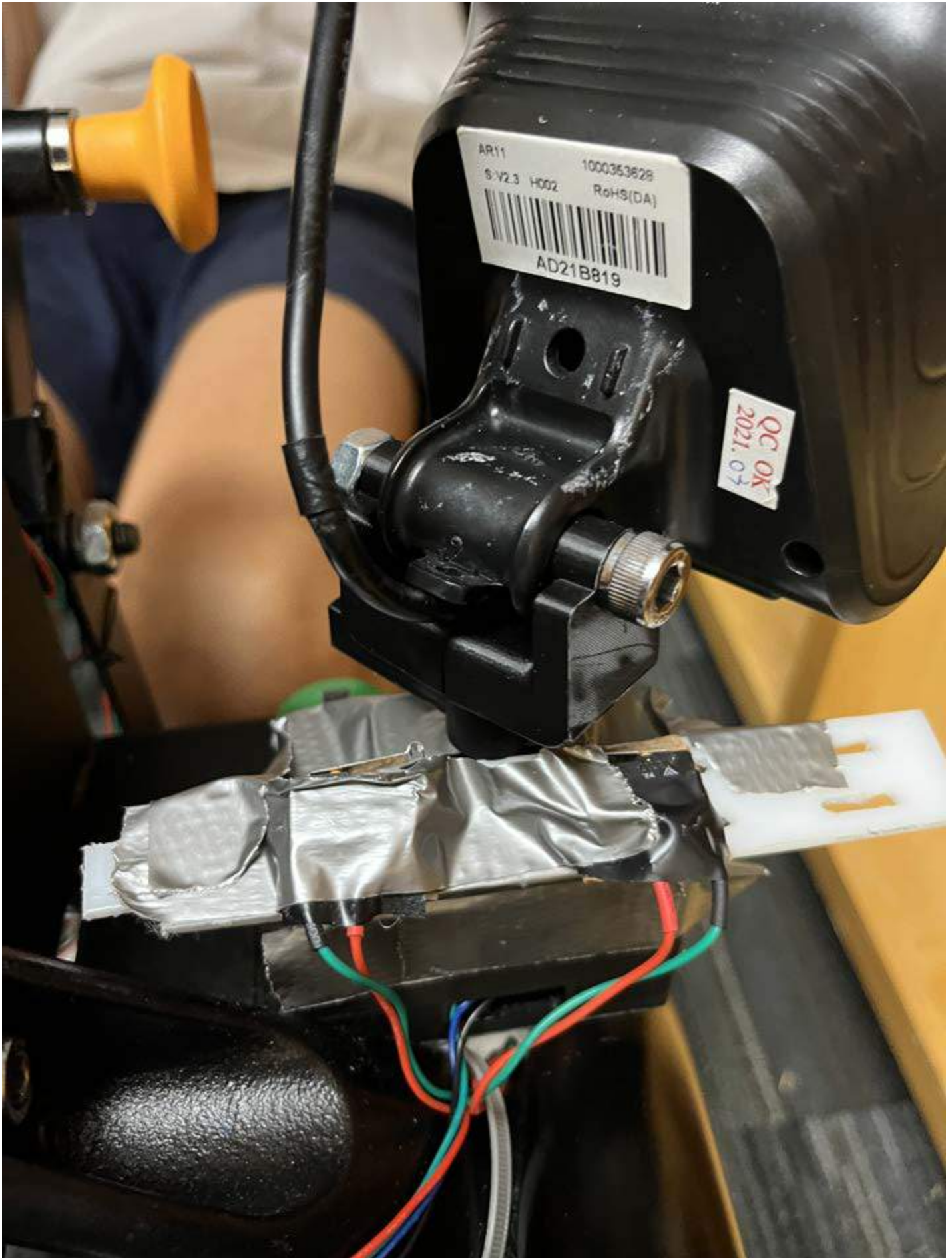
The above image shows the limit switches and console connected together.
