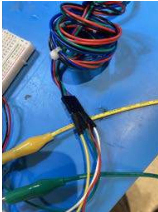
IMG_6988.jpeg (1.88 MB) Image showing motor connections. Blue and green are one coil and red and blue are the other coil.
