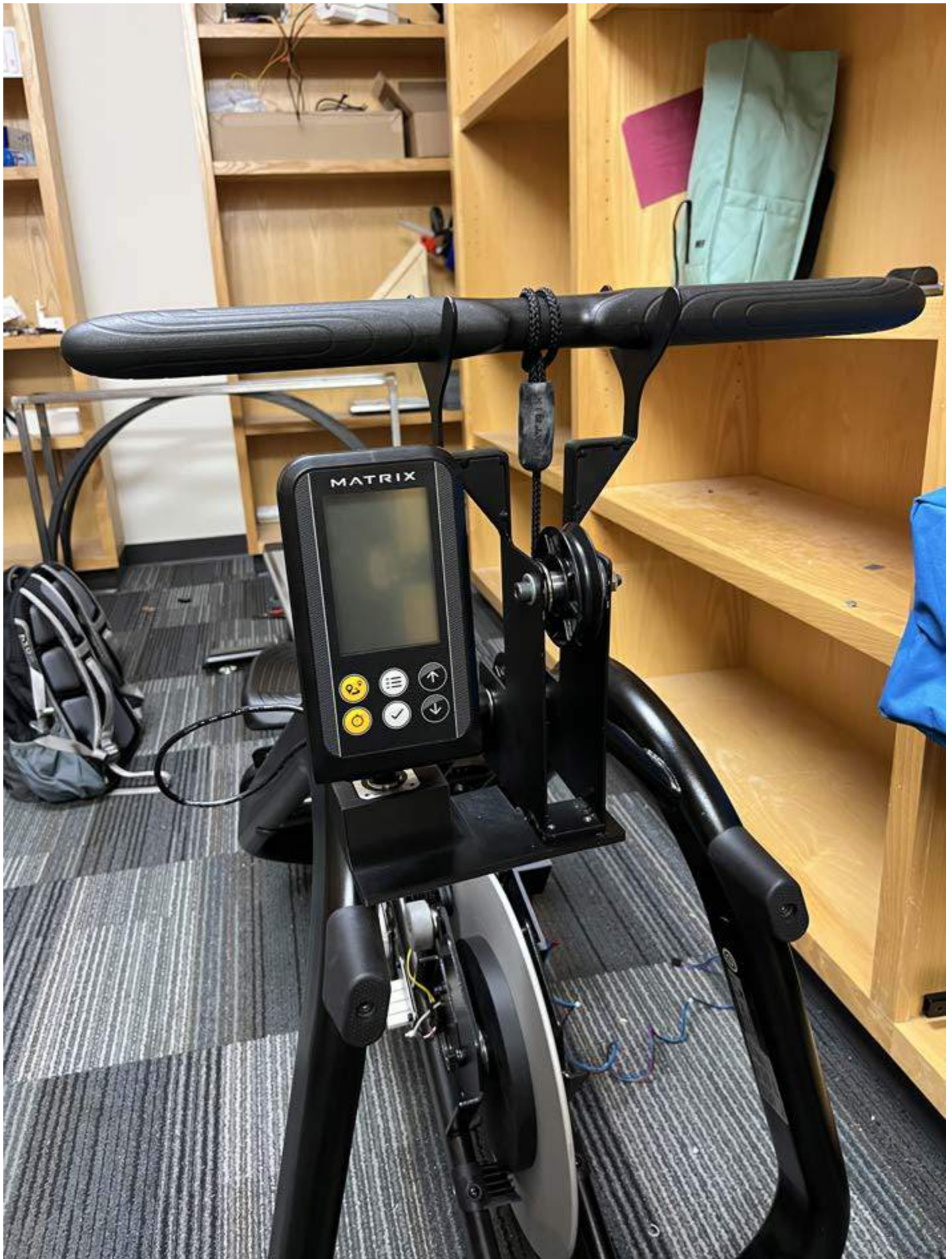
The above image shows the front view of the console box secured to the metal pulley plates.
