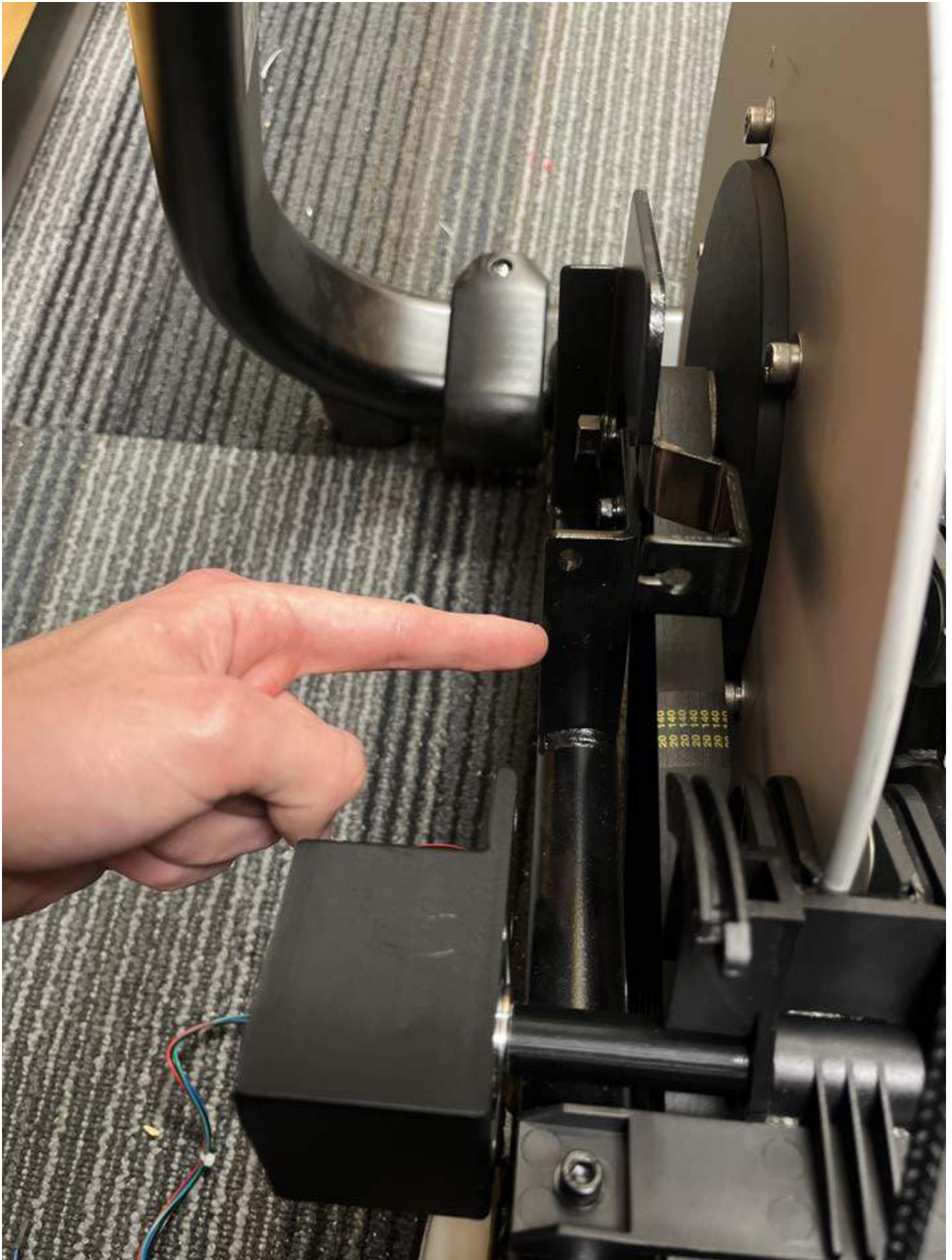
The above image shows the flat edge we will screw the motor housing into.
