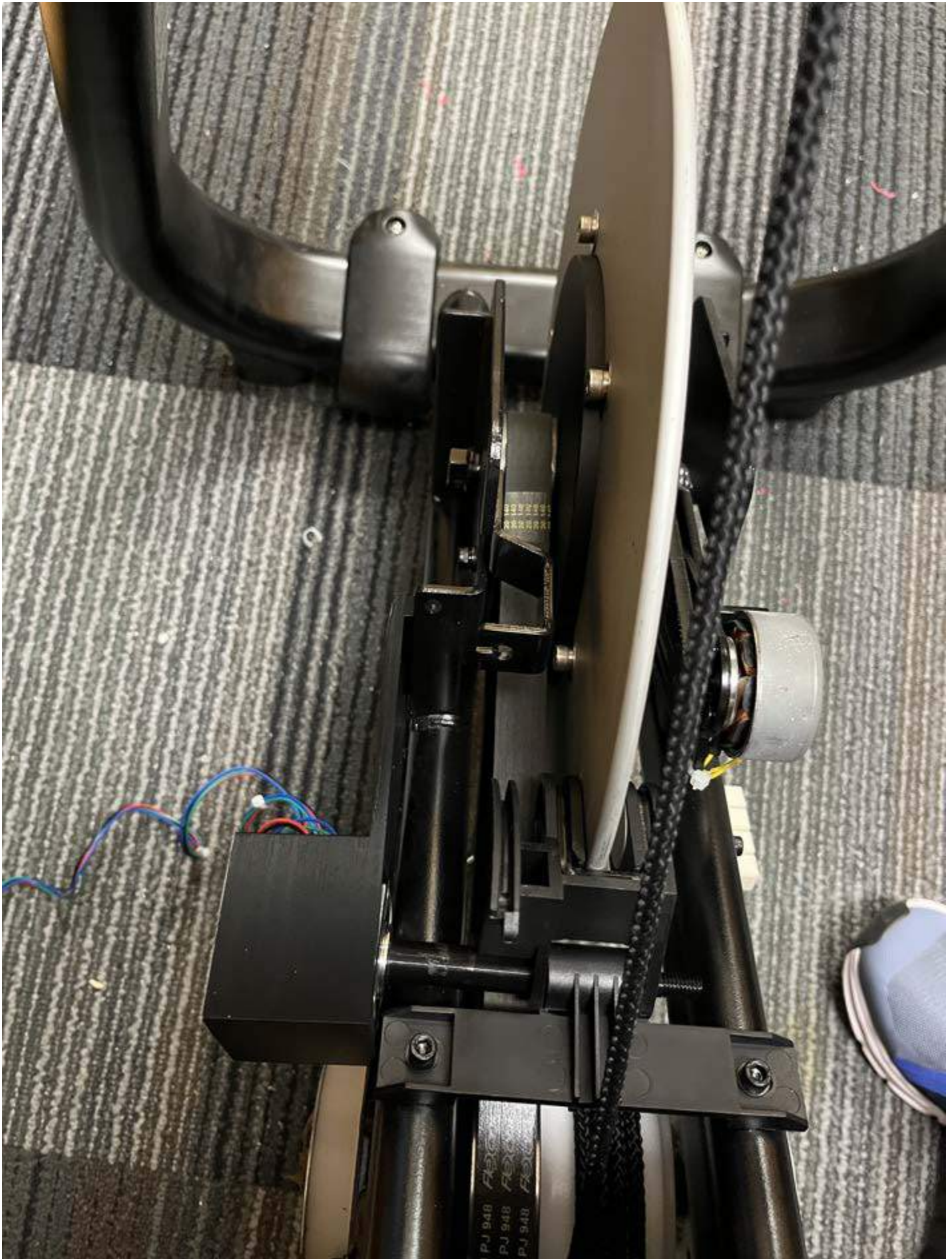
The above image shows how the new motor housing will screw into the rower flat edge.
