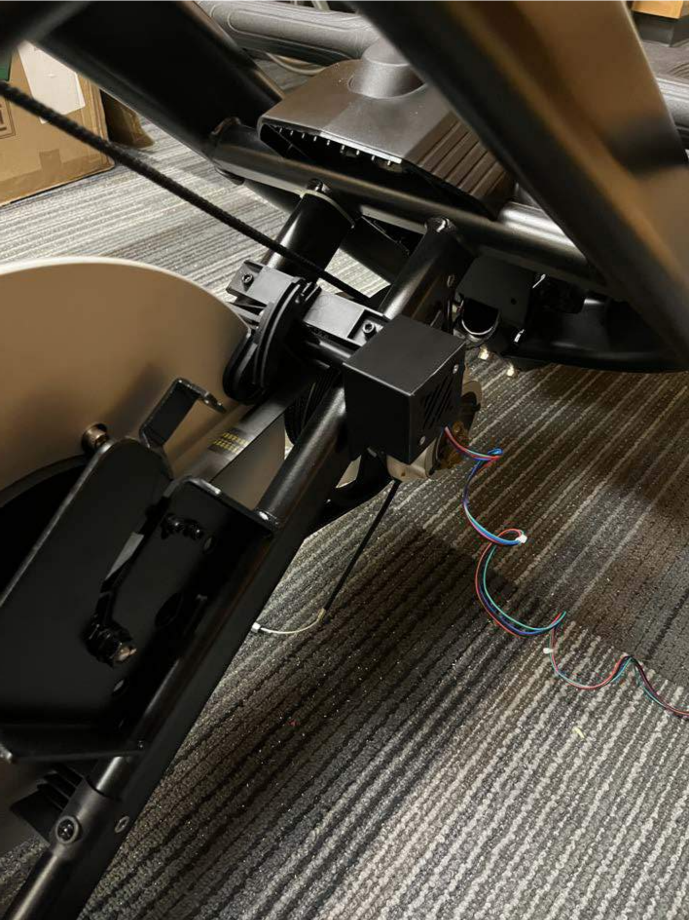
The above image shows the top view of the newly proposed motor location when the magnets stay in their original location.
