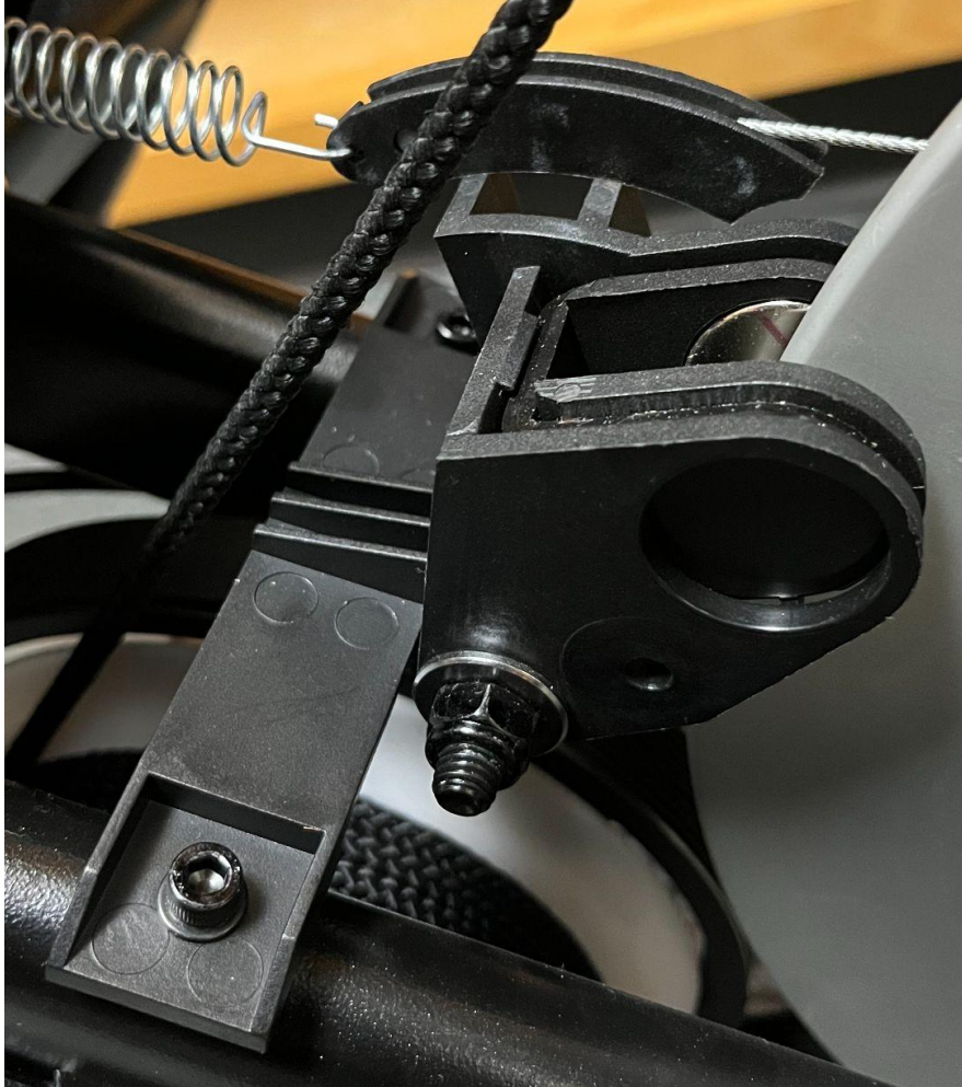
Figure 4. Current location of magnet housing. The magnet housing is currently screwed into the support portion of the two angled support bars that are within the plastic housing of the rower. The housing is one large piece of plastic that rotates about the central bolt shown above. The proposed resistance dial mechanism will keep this entire structure intact, but move it to another location within the inside of the rower.
