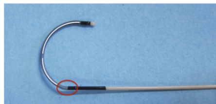
Fig. 7 Inhomogeneous bending of the tip for a 180 deg angle. A sharp bend was observed at its base (red circle), and the proximal and distal part of the tip presented two radii of curvatures (white arcs of circle drawn over the tip).
