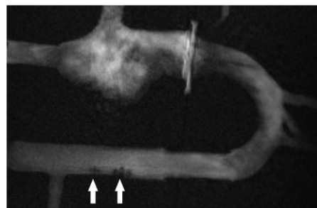
Fig. 9 MRI scan (fGRE RT, slice thickness 12 mm (0.047 in.), 1 fps) of the steerable guidewire in a vascular model (transcatheter valve simulator heart model, Elastrat, Geneva Switzerland) with pulsatile flow. The two passive markers (white arrows) indicated the localization of the steerable tip that was lying in the thoracic artery, above the celiac trunk.
