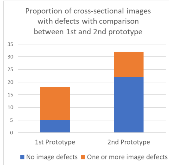
Figure 6.D2. Proportion of cross sectional images with defects as compared between 1st and 2nd prototype. More images were taken for the second prototype. 27% of images had no defects for 1st prototype and 69% of images had no defects for 2nd prototype.
