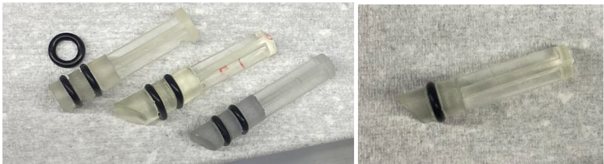
Figure 5.4. Design progression of plungers. From left to right: flat end, 30 deg ramp, 40 deg ramp (prototype 1), single O-ring 40 deg ramp (final, prototype 2).
