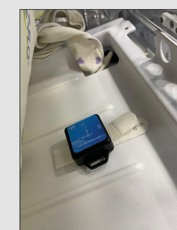
Figure 11: Placement of WitMotion accelerometer inside the inner tray. Secured with two command strips.
