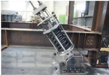
(a) Spring viscous damper
