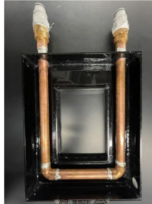
Figure 24: Top view of the new incubator box showing the caulking and copper piping
