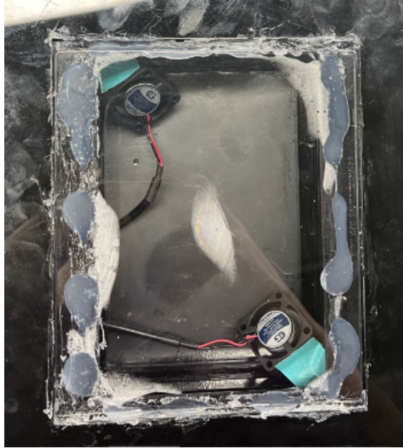
Figure 6: Photo showing the opposite corner dual mini fan setup where the fans are angled up at roughly 45 degrees
