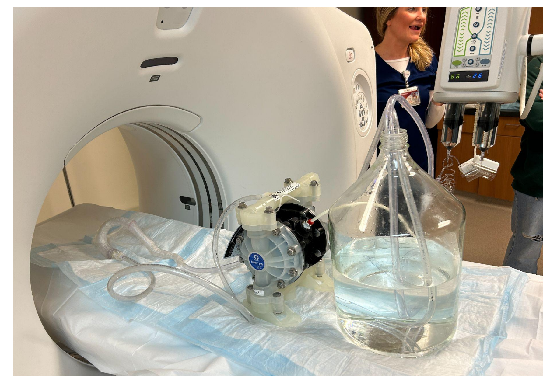
Figure 6: Circuit on the CT table prior to scanning.
