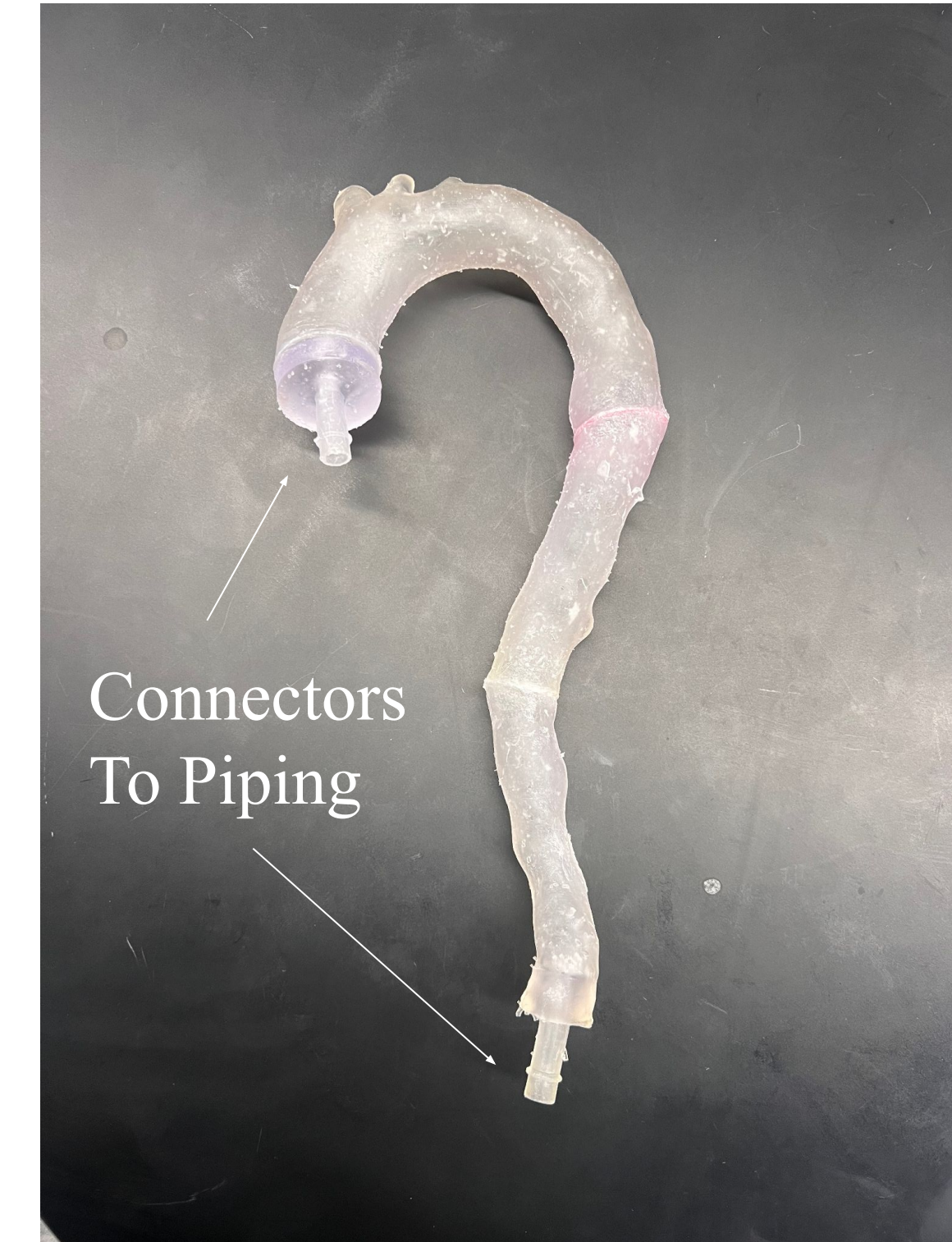
Figure 4: Elastic 50A Resin 3D printed Aorta phantom.
