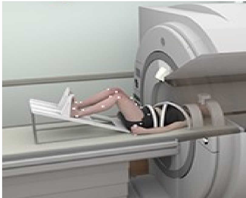
Figure 1. Emory University illustration depicting their bilateral hamstring activation device and overall experimental setup with fMRI [6].
