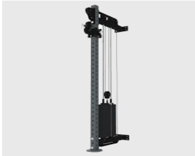
Figure 12. Representation of the cable stack design. Important features of the design include the pulley system to move the weights as well as the supports [30].
