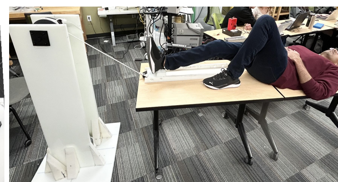
Figure 12. Side view of fully assembled leg loader with subject
