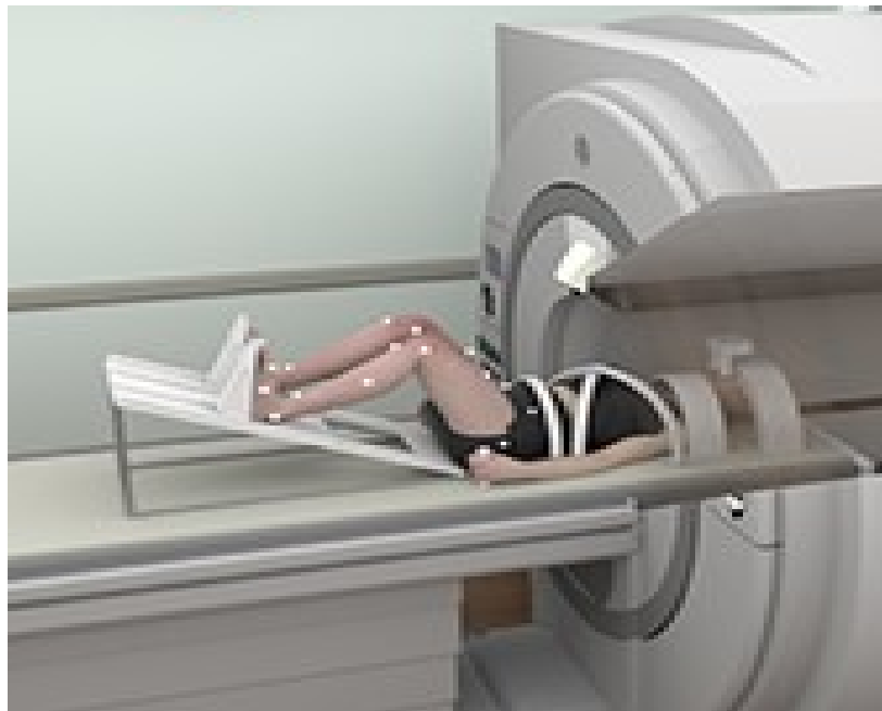
Figure 1. Emory University illustration depicting their bilateral hamstring activation device and overall experimental setup with fMRI [6]. See also the motion capture optical markers and contraption to secure the upper body.
