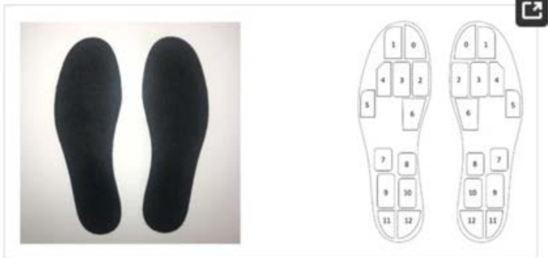
Figure 2. Moticon insoles and the number of sensors covering the insole area (not to
