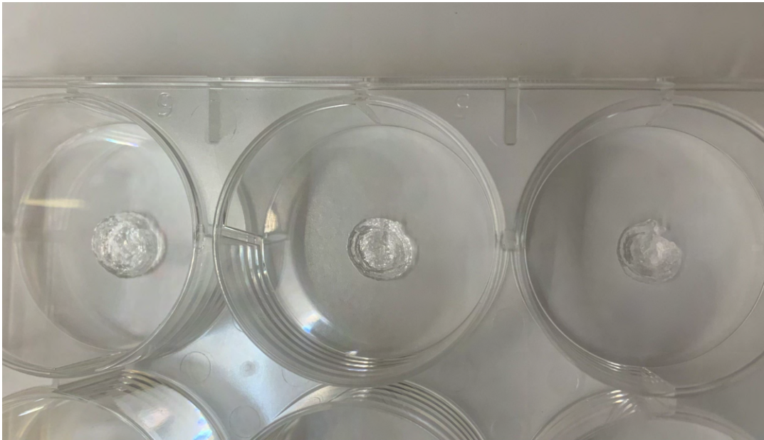
Figure 2: Top view of print 2. Loss of structural integrity on the third gel off this print, observed to likely be due to an increase of viscosity in the GelMA as the print progressed.
