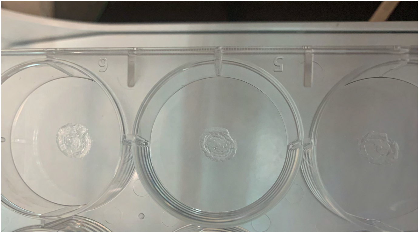
Figure 3: Top view of print 3. The concentric pattern structure looks good, but the thickness of these gels suggests that insufficient volume was being dispensed during this print (see figure 4).
