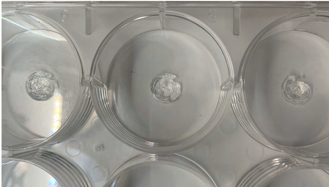
Figure 3: Top view of print 3 of the day. All three gels have consistent structure in the middle, but start to lack volume on the outer edges. There appears to be gapping occurring between concentric filaments.
