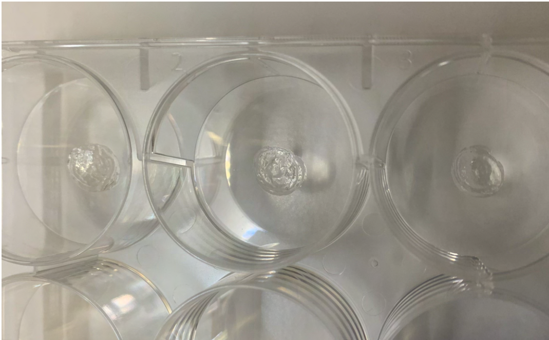
Figure 1: Top view of print 1. All three gels printed with structures lacking gaps, but diameters exceed 10 mm.
