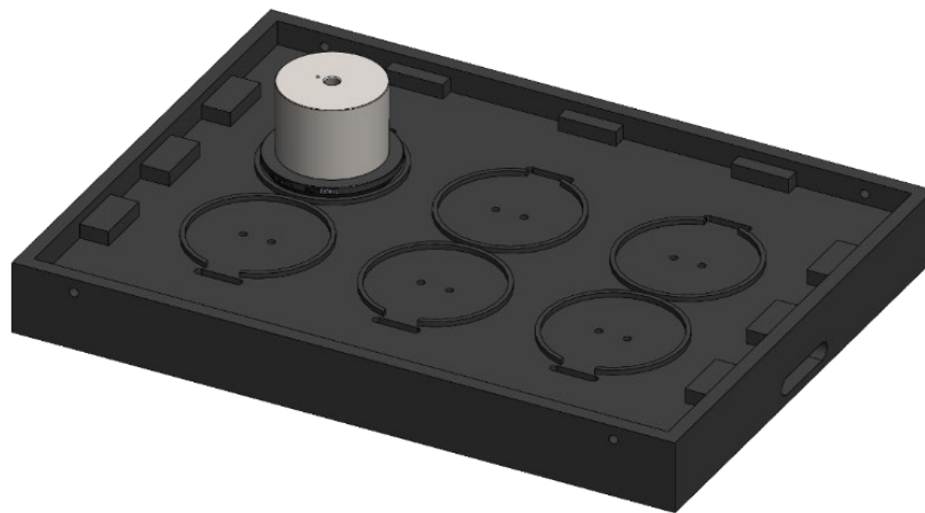
Figure 5. Trimetric view of the sample base, with one VCA included for reference.
