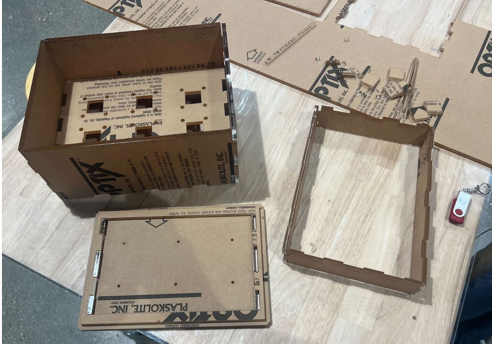
Figure 16. Quick assembly of the bioreactor's acrylic panels to demonstrate their compatibility immediately after cutting.
