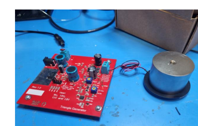
Figure 5. Setup to control VCA with triangle voltage generator PCB
