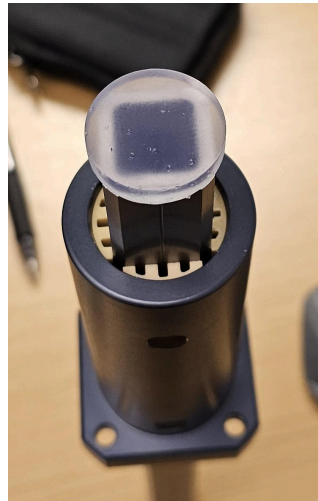
Figure 6: Press-fit plunger (i.e., which will contact the sample dish).
