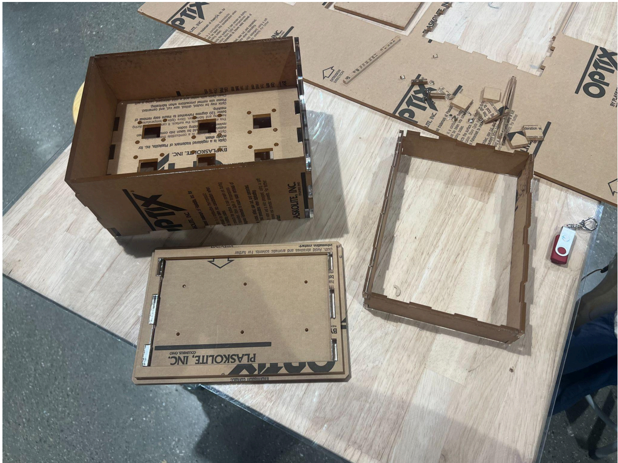
Figure 2: Testing the tongues and grooves of the cut acrylic pieces to see how they fit together (no adhesive has been used yet).
