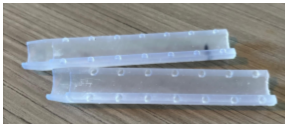
Figure 1: Image of 3D printed coring device opened to allow tissue to be removed.
