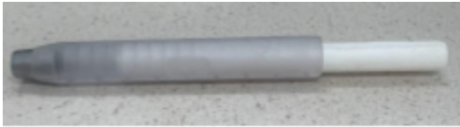
Figure 3: Final assembly consisting of blade, coring tube, and plunger.
