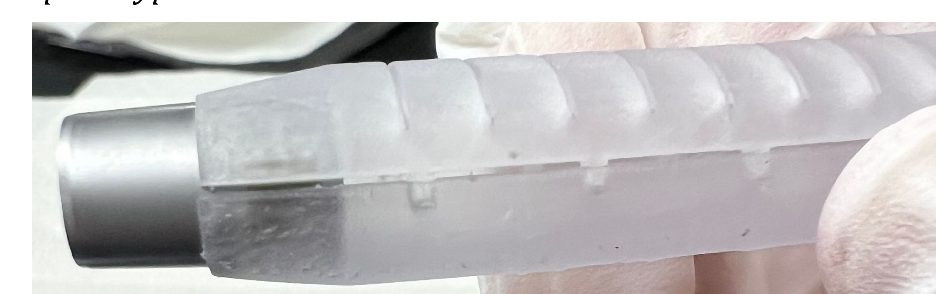
Figure 14: Close up of Tube #13 showing the gap created when too much force from blade.
