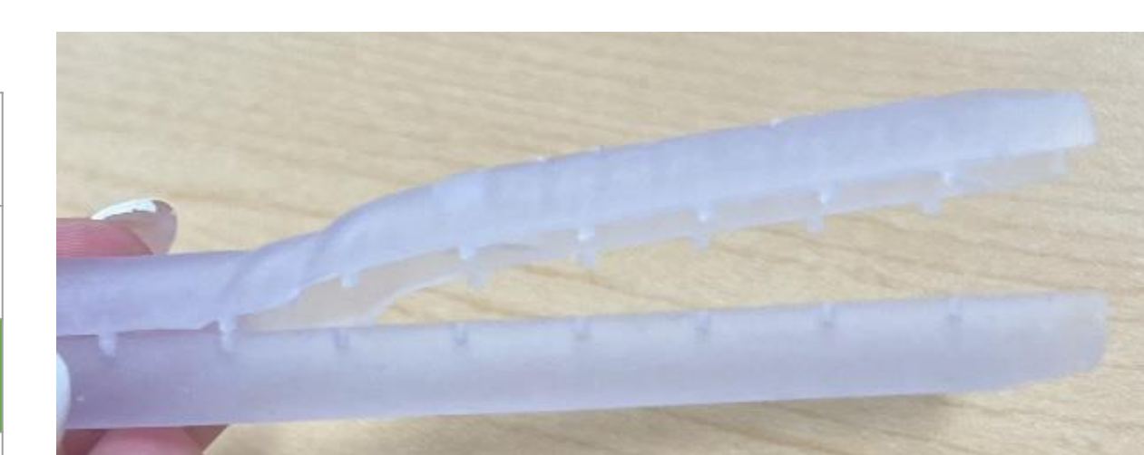
Figure 16: Coring tube deformed after being UV cured at 60 C for 15 minutes.
