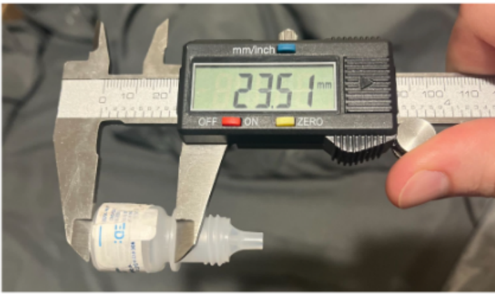
Figure 4: ~23.51 mm from cap base to bottle base for glaucoma bottle.
