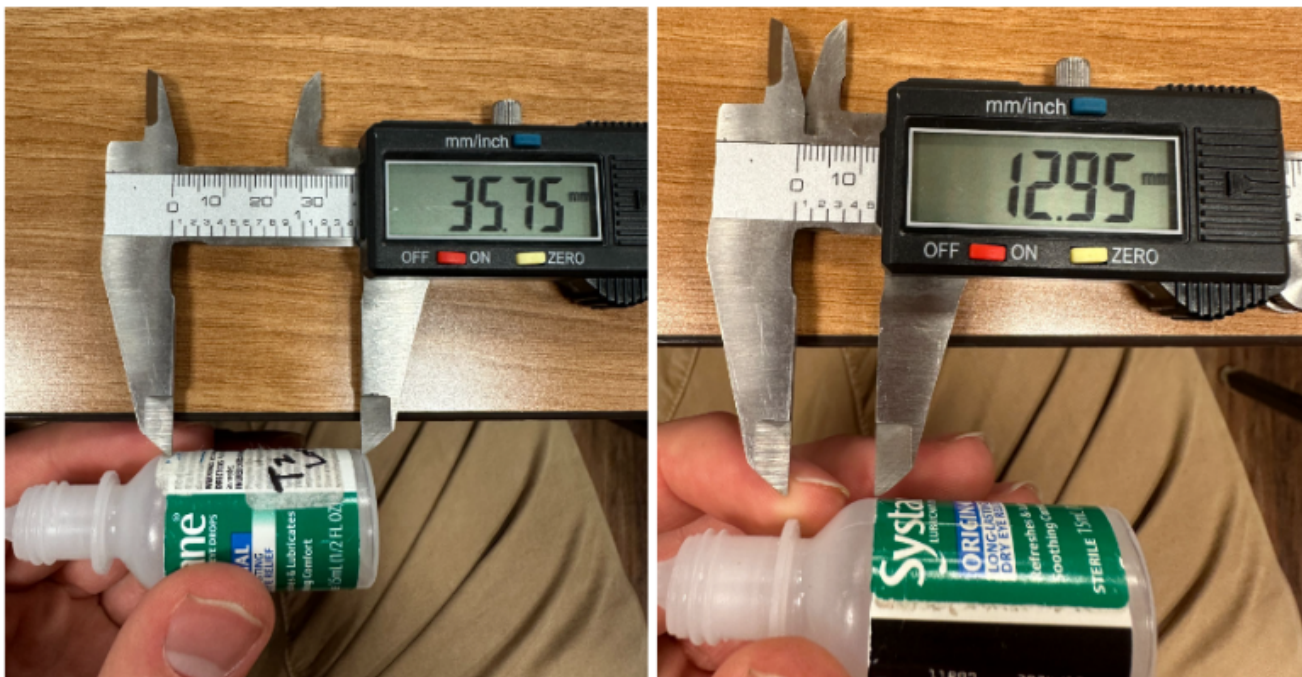
Figure 1: ~48.7 mm from cap base to bottle base for Systane bottle.
