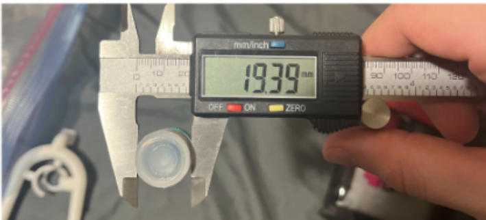
Figure 5: ~19.39 mm is the maximum width of the glaucoma bottle
