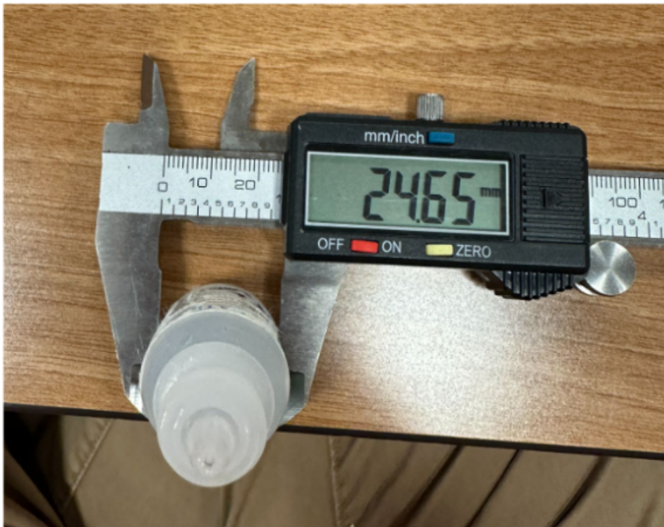
Figure 2: ~24.65 mm is the maximum width of the Systane bottle
