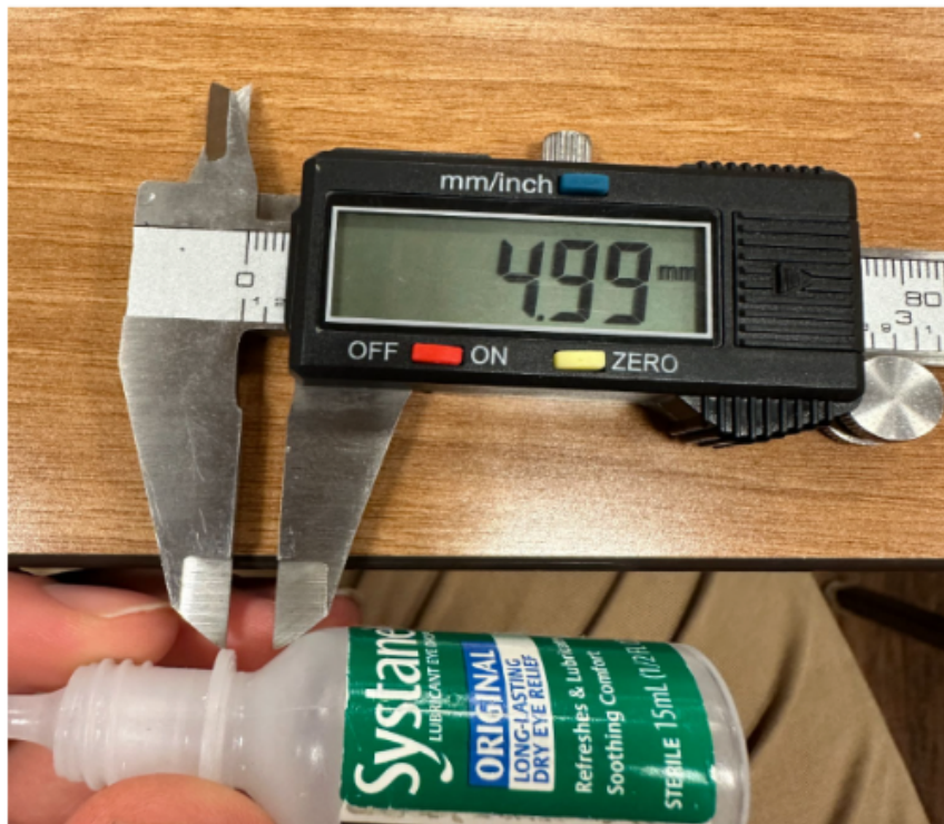
Figure 3: ~4.99 mm from cap base to the start of bottle curve for the Systane bottle
