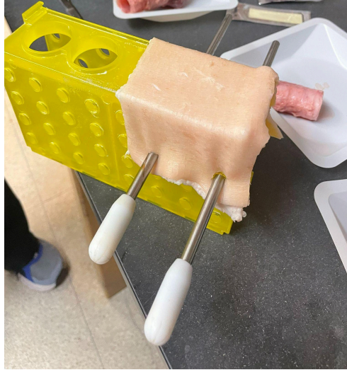
Figure 2: Affixation of porcine skin apparatus
