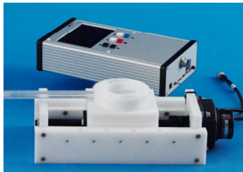
Figure 4 Vital Biomedical Technologies MRI Compatible Motion Stage [13]
