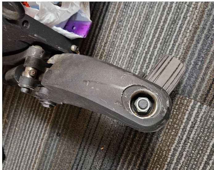
Figure 3: Bolt hole that the castor cap slots into
