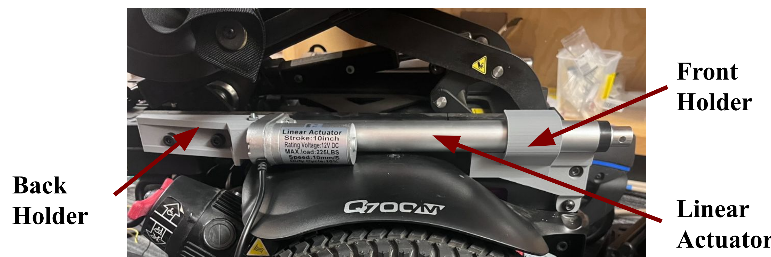
Figure 4. Linear actuator support/attachment to wheelchair
