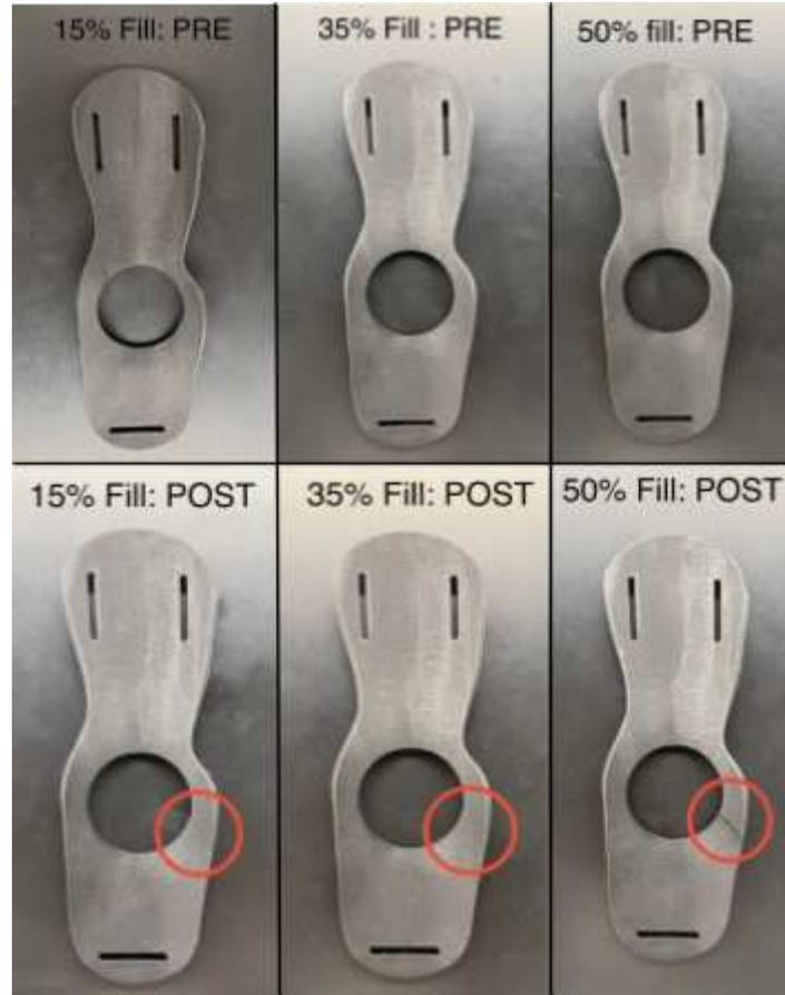
**Figure 22:** Pre- and Post-MTS Testing Samples.
