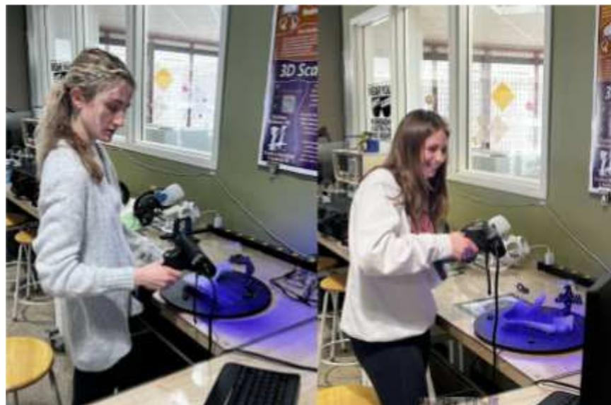
**Figure 17:** 3D Scanning of Cast using Creality Raptor X.
