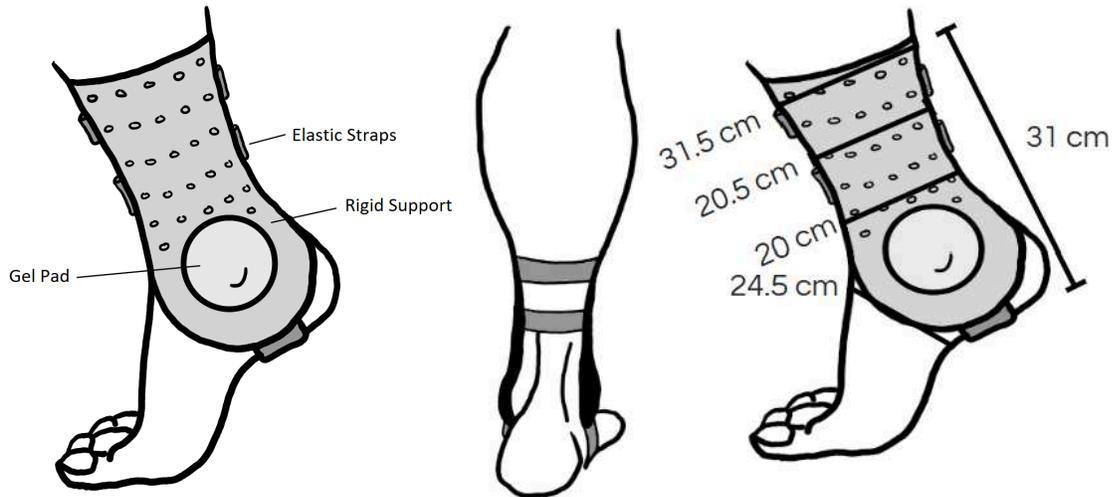
**Figure 11:** We Support U Dimensions and Components.
