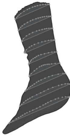
13. Using the "loft" tool, connect the sketches in the order they appear on the cast.
