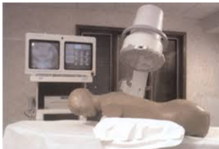
Figure 5: RSD Needle Placement Phantom from Supertech to visualize what a phantom looks like [28].
