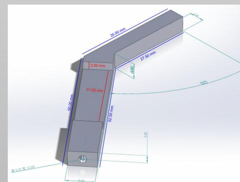
**Figure 4:** SolidWorks model for the prongs of the device.
