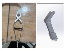
A preliminary CAD model was developed with SolidWorks and printed at UW-Madison Makerspace. Then a test tube holder was cut to fit. After that, a hole was drilled into the plastic pieces and hot glued onto the metal. Foam was also hot glued onto the end.
