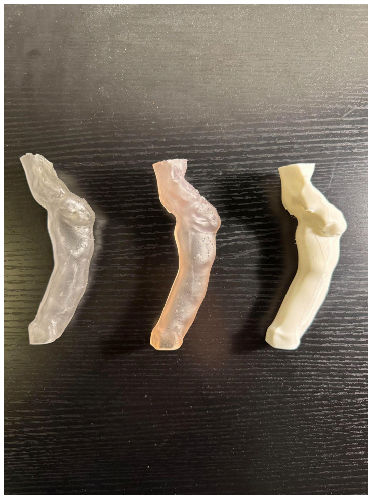
Figure 6: Three Printed Airways, Material from left to right: Elastic Resin, Flexible Resin, TPU MRI & Segmentation
