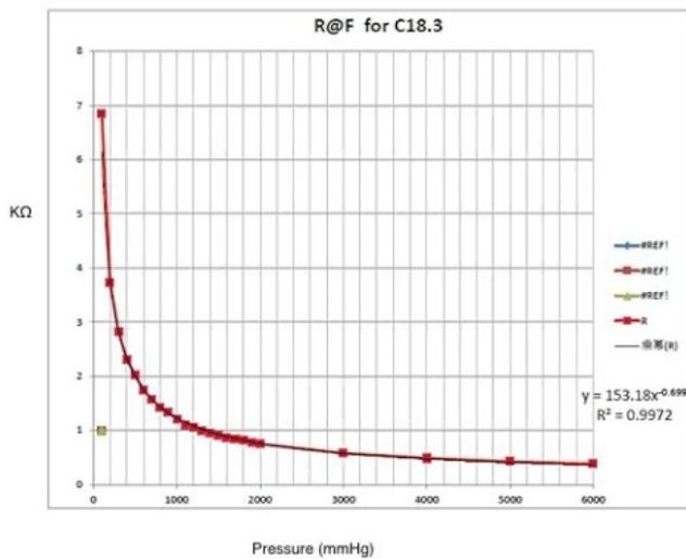
$Y = 153.18 \times X^{-0.699}$  where Y is resistance in KOhms and X is pressure in mmHg
