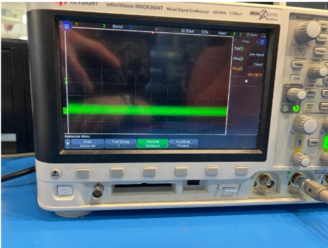
This figure is obtained by using two different inputs: 150 and 200 mV, as inputs. This is observed at the output of the voltage follower.
