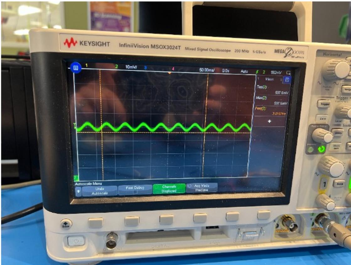
This figure is the output observed at instrumentation amplifier. All common mode signals are rejected.
