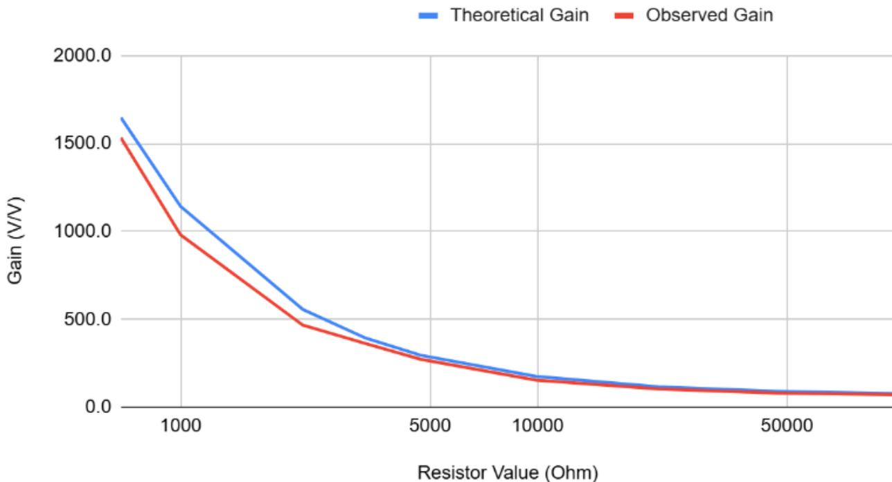
The chart below shows the absolute percent error of the observed gain from the theoretical gain. The percent error is consistent with an average of 11% and a standard deviation of 3%.
