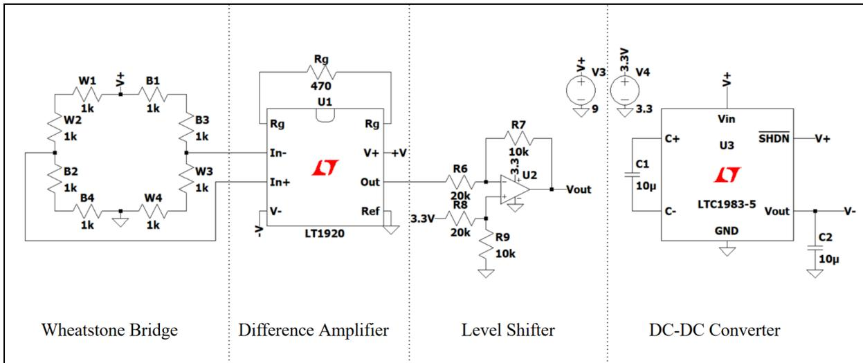
Figure 2. Circuit diagram of the load sensor amplifier. From left to right, the Wheatstone bridge of load sensor, with each node representing a load sensor embedded within each leg, LT1920 (U1), level shifter (U2), and LTC1983-5 (U3) constitute the load sensor amplifier.
