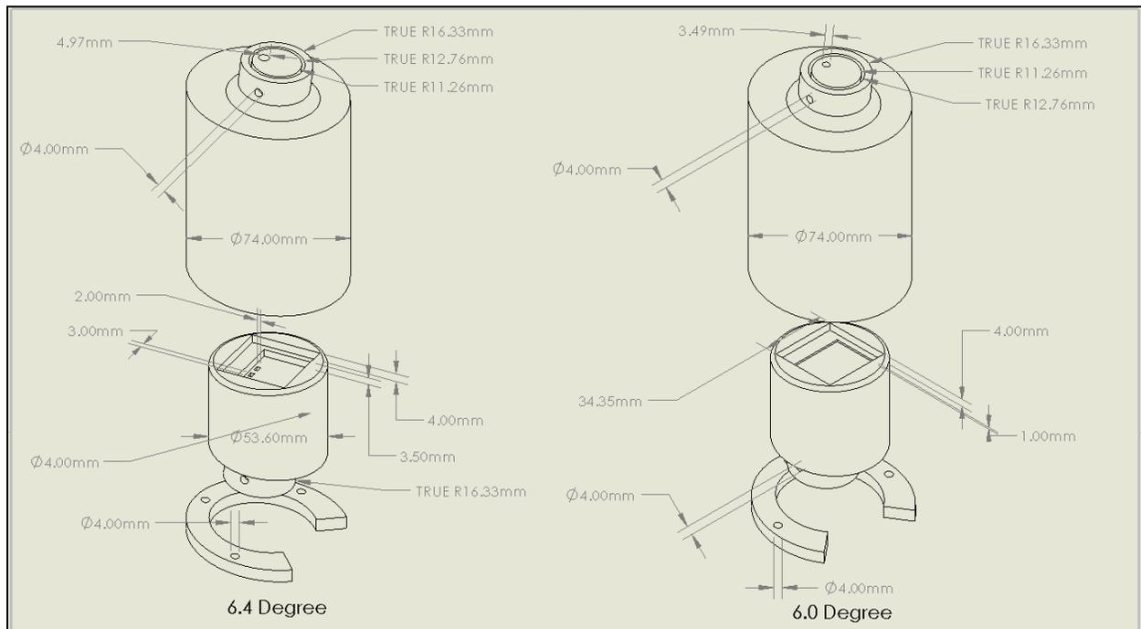
Figure 6. Annotated Solidworks drawing of the Load Sensor Holders (mm).
