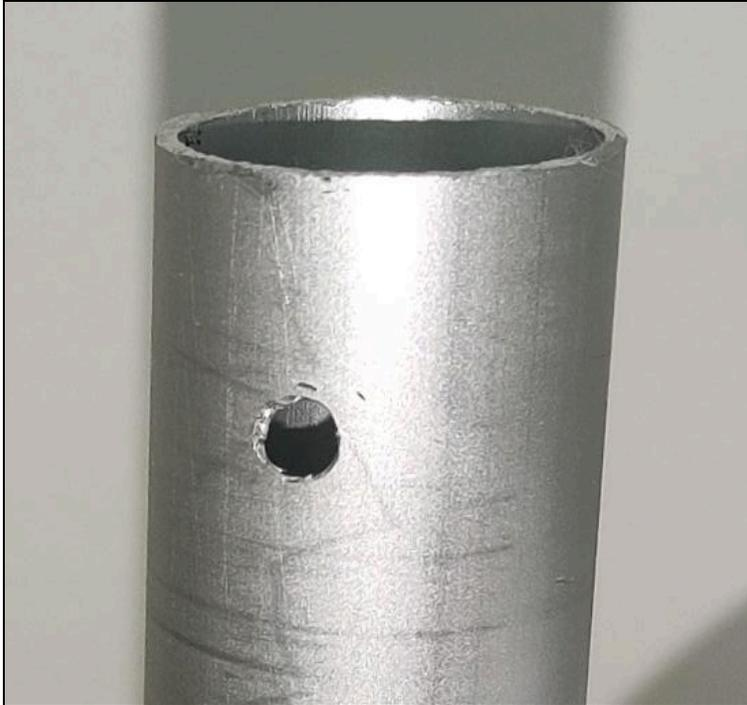
*Figure 10. Bolt hole for the load sensor holder.*
