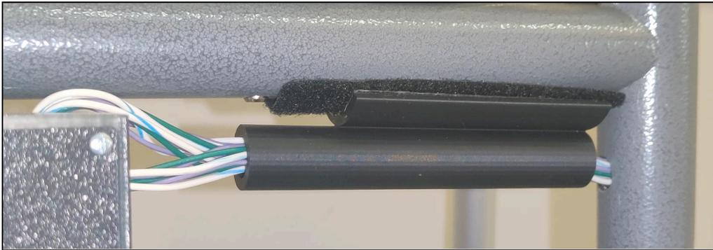
*Figure 13. Upper wiring leaving the walker frame and travelling through a wire conduit before entering the electrical housing on the left.*
