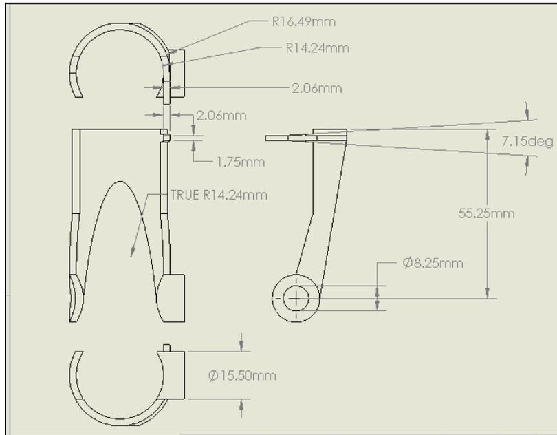
**Figure 9. Infrared sensor holder CAD and dimensions (mm).**
