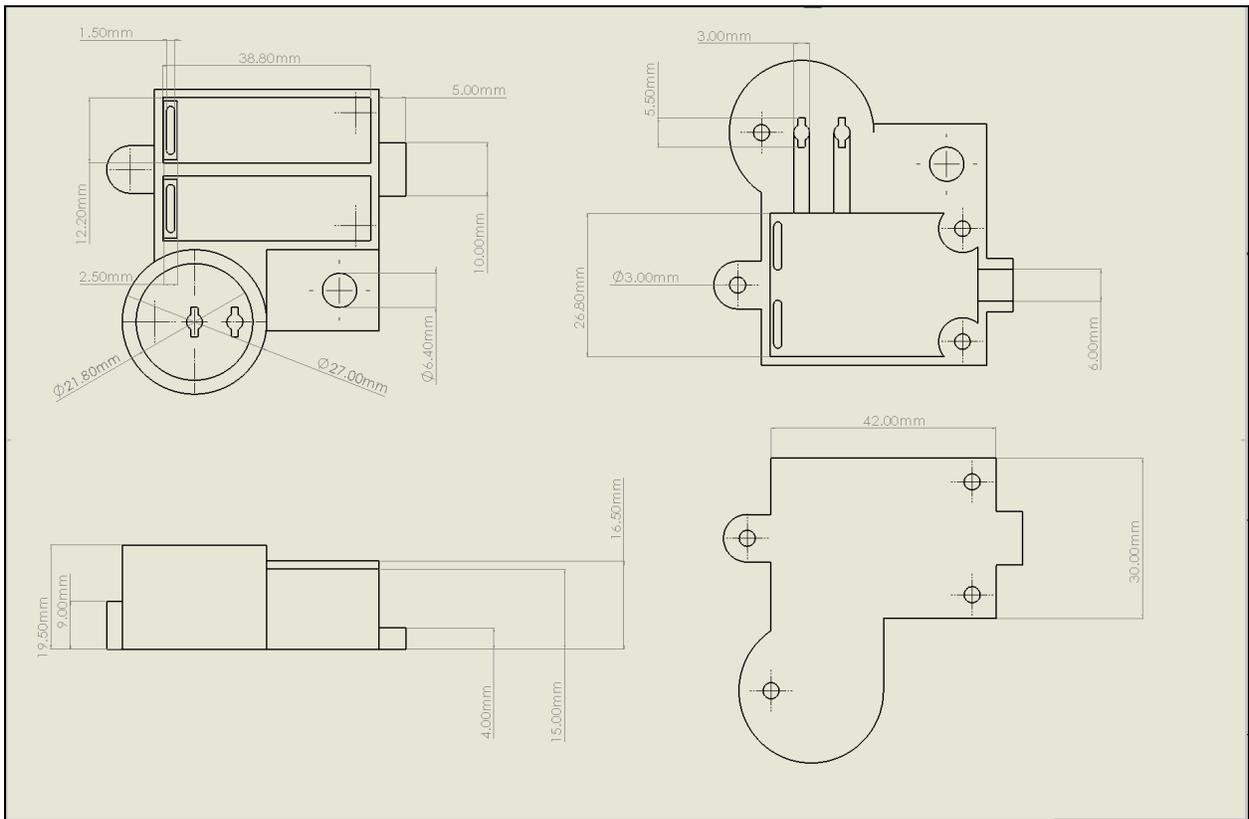
Figure 8. Display and trial switch holder CAD and dimensions (mm).
