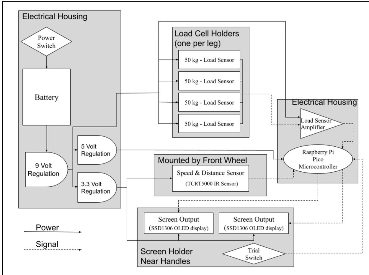
Figure 1. Block diagram of smart walker design and components. This schematic shows the power and signal connections between components, as well as the relative position of each component on the smart walker.
