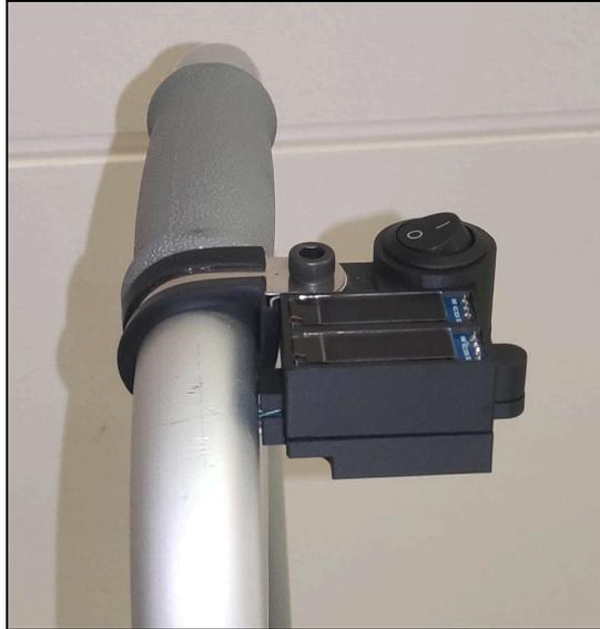
Figure 17. The mounted screen holder on the left handle with the two OLED screens and trial switch within the component.
