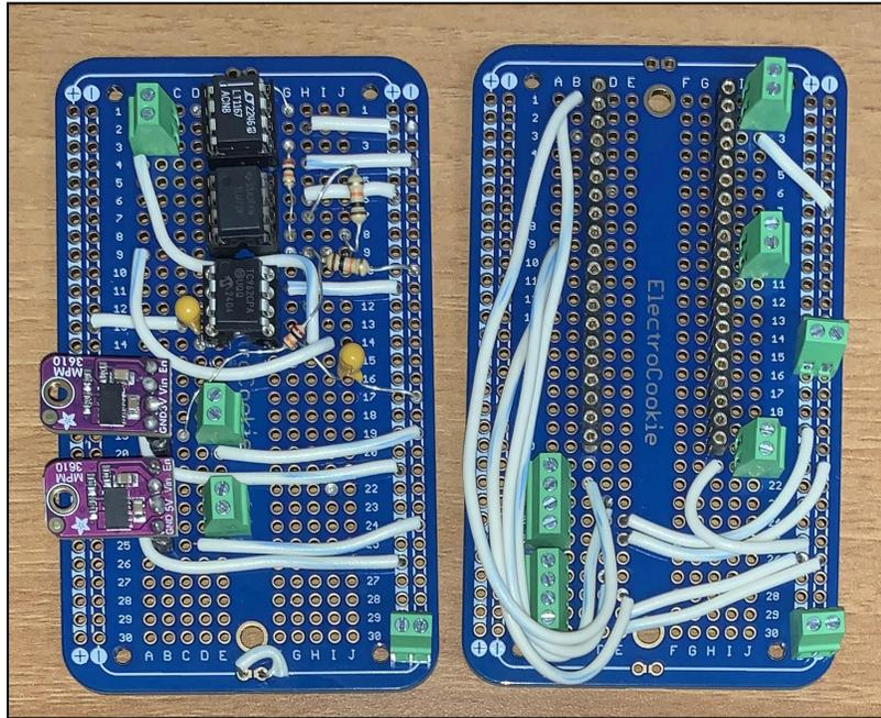
*Figure 14. Image showing soldered connections made on each of the breadboards.*
