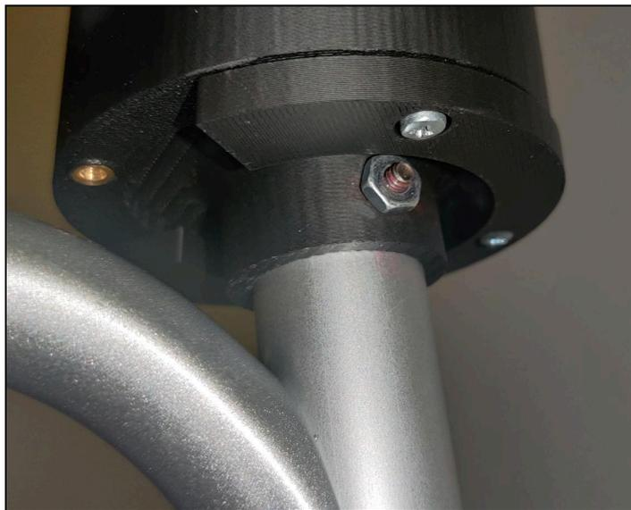
*Figure 16. C-ring that connects the bottom and top components of the load sensor holder.*
