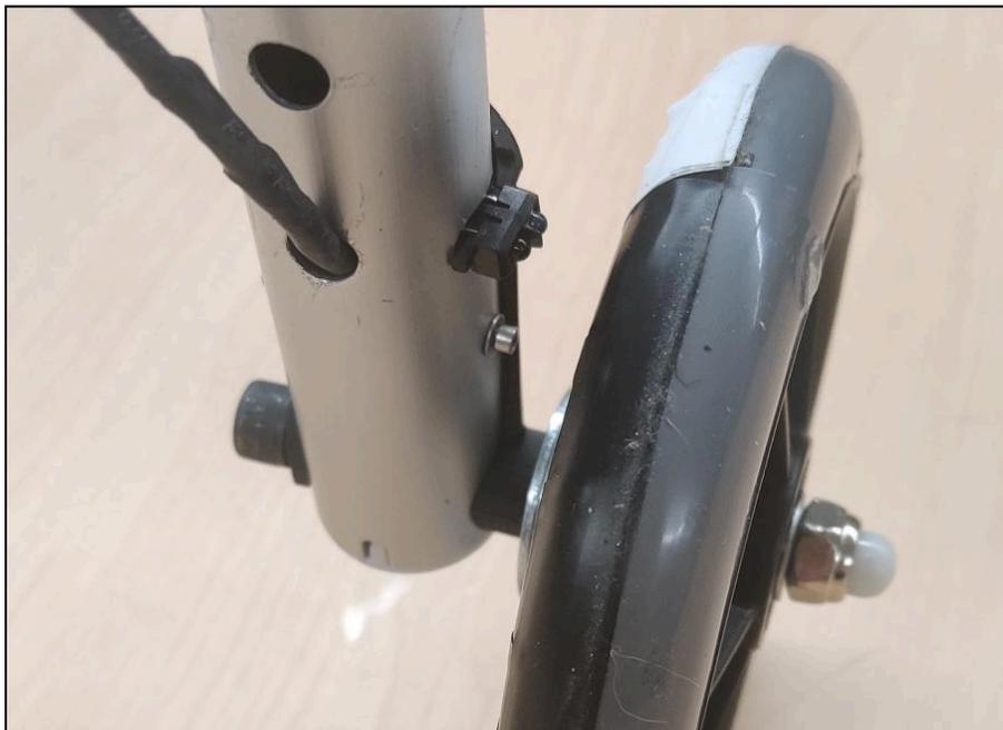
*Figure 15. Mounted IR sensor and holder.*
