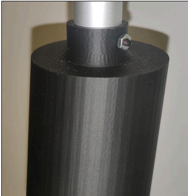
*Figure 11. Bolt hole for a top load sensor holder.*
