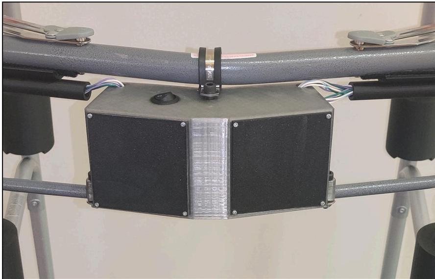
*Figure 12. Image showing the electrical housing, and how it is mounted to the smart walker, along with how the wires feed into the housing.*
