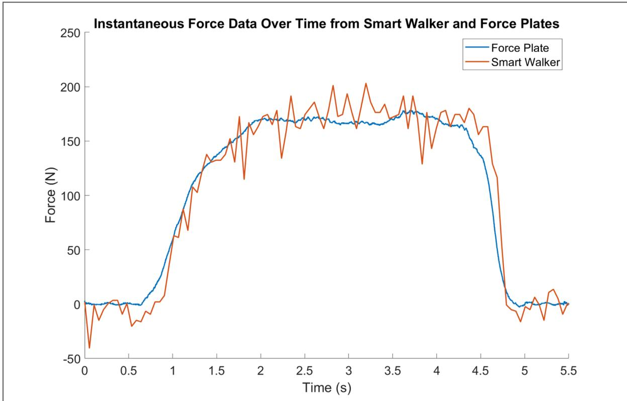
*Figure 5. Measured applied load (N) comparison between in-ground force plate data (N) over time for one trial.*
