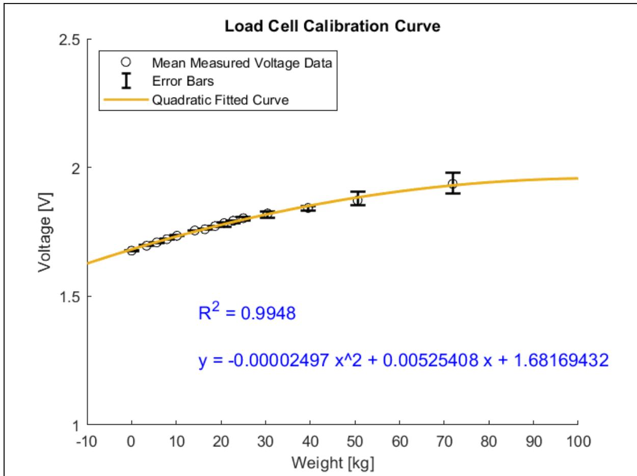
Figure 4. Calibration curve of weight applied (kg) and output voltage (V).
