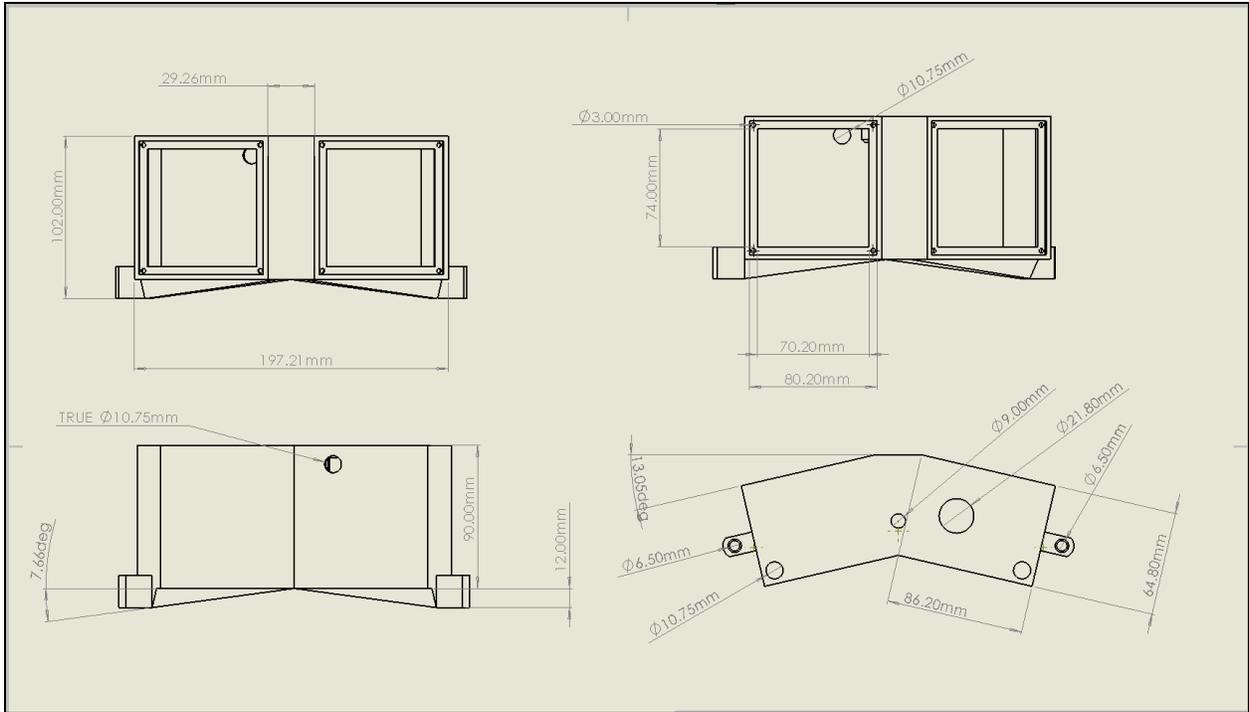
Figure 7. Power and Sensor Circuitry housing CAD and dimensions (mm).
