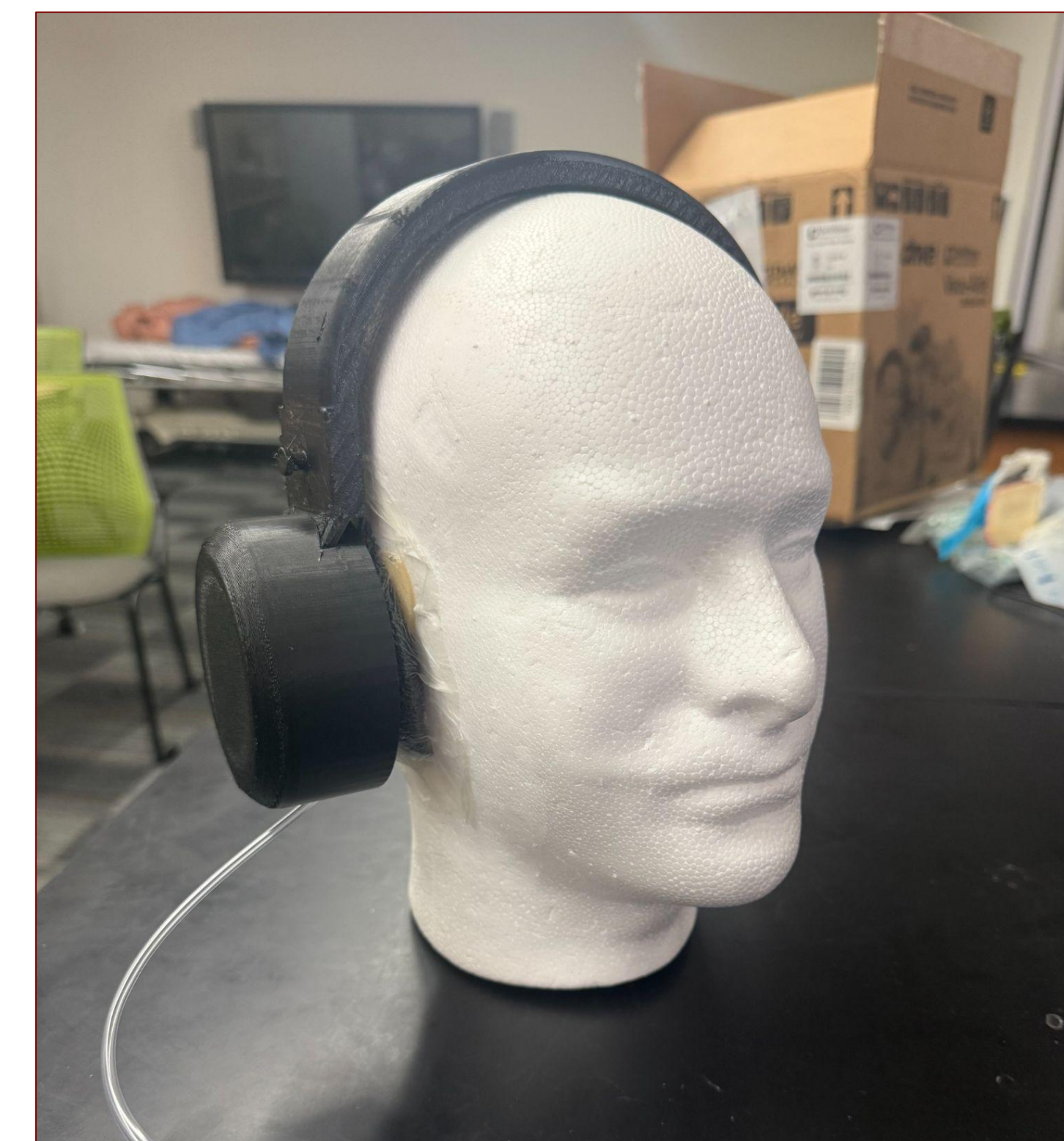
Figure 5: The earmuff / headphone piece situated on a model while negative pressure is applied
