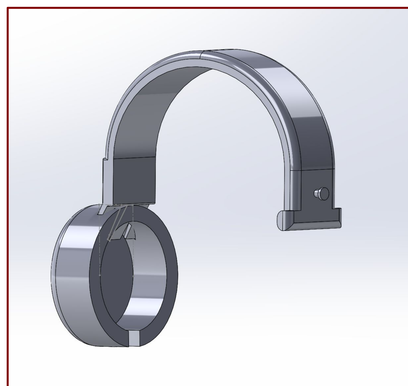
Figure 4: SolidWorks model of final design, interior of earmuff included
