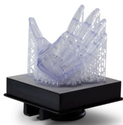
Figure: hand model printed out of Flexible 80A Resin
