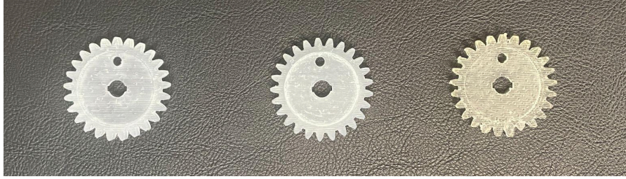
Figure 7: The three IRE materials tested: Control (left), Sanded (center), and Flexible (right)
