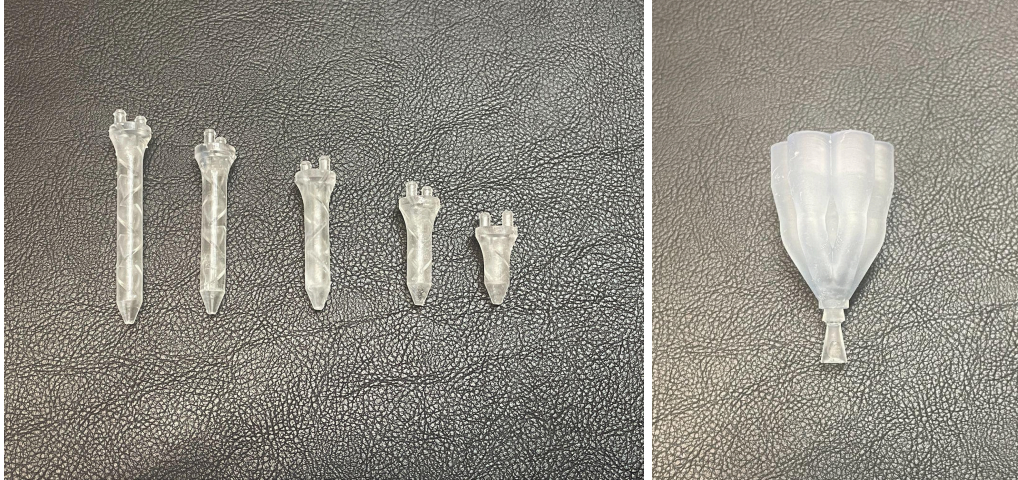
Figure 1: Five of seven different sizes of KSM, from 1 to 5 mixing elements (left) and a CEVIC (right)
