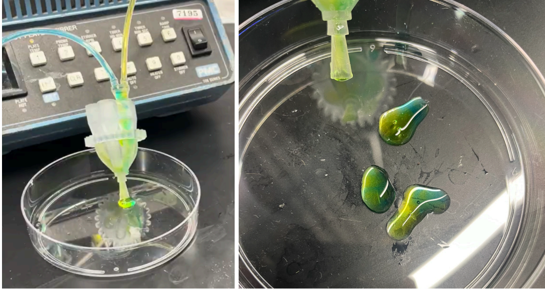
Figure 9: Testing pushing two different colored gelatins through the CEVIC and IRE (left) and the resulting hydrogels (right)
