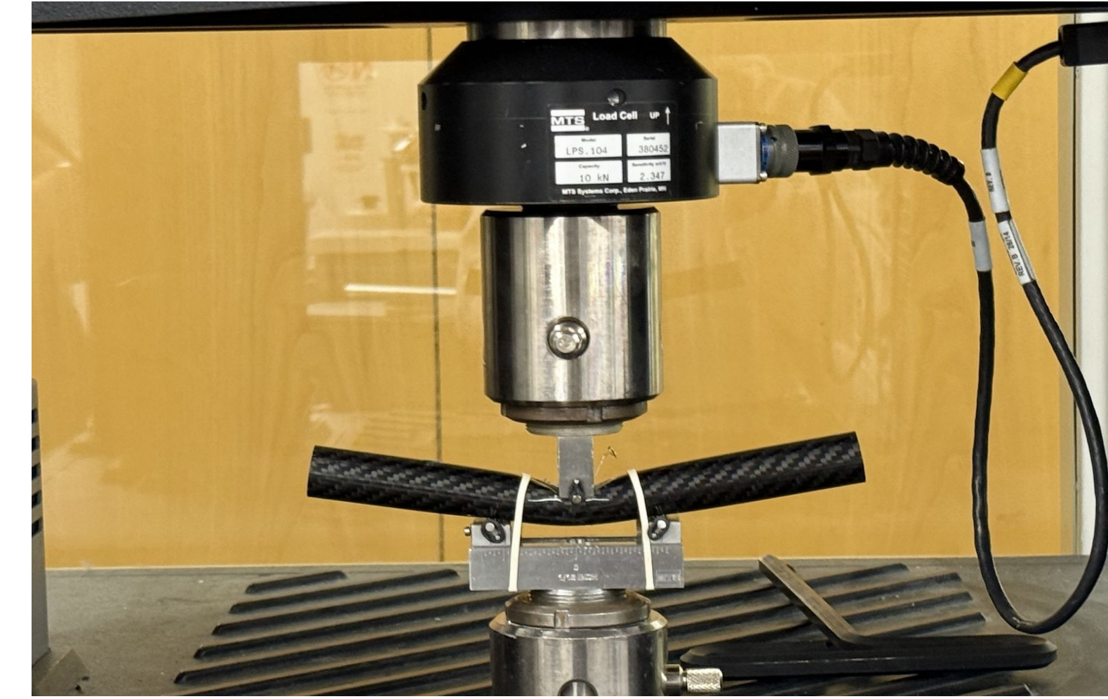
Figure 11: Carbon fiber rod during 3-point bending MTS testing
