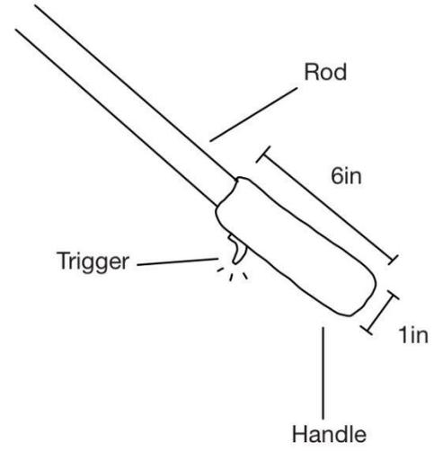
Figure 7: Manual Trigger
