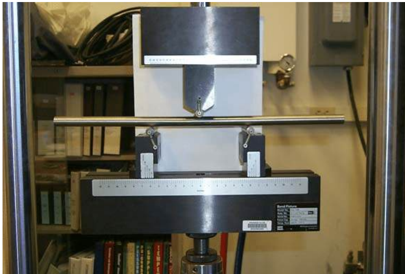
Figure X: 3 point bending in an MTS machine [X]
