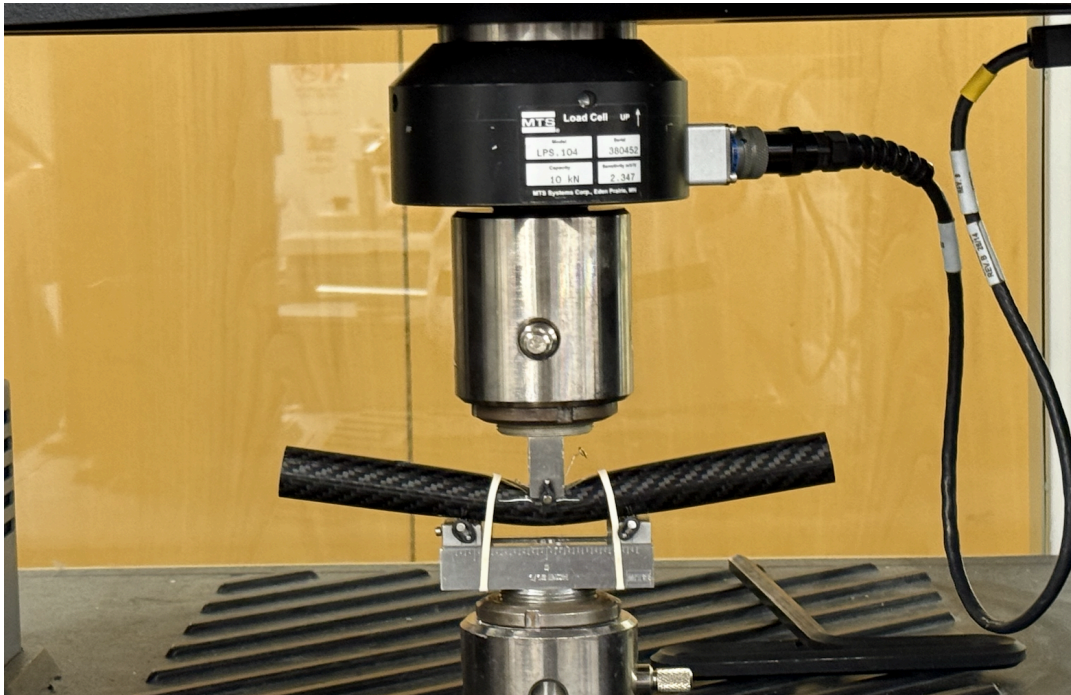
Figure 19: MTS 3-point bending setup
