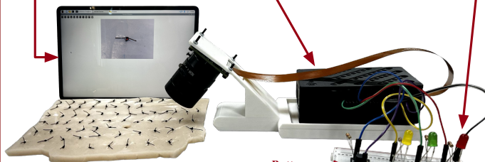
Figure 6: Overall system setup showing HQ camera, Raspberry Pi, and breadboard hardware. User input via button initiates a camera preview. Second click initiates image capture that is passed through the model (housed on the Pi) and model output indicated by red and green lights.
