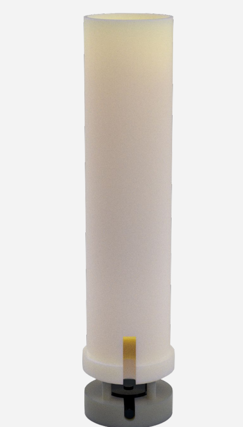
Figure 5: 3D printed disk to hold load cell
