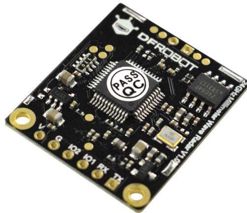
Figure 7: mmWave Radar Sensor with dimensions of 24 x28mm[13]
