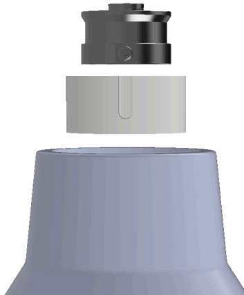
Figure 8: CAD design of the integrated end-cap design. The design included three separate sections with the base having dimensions of (30mm), the middle section having dimensions of (24mm), and the top section having dimensions of (25.4mm x 30mm)
