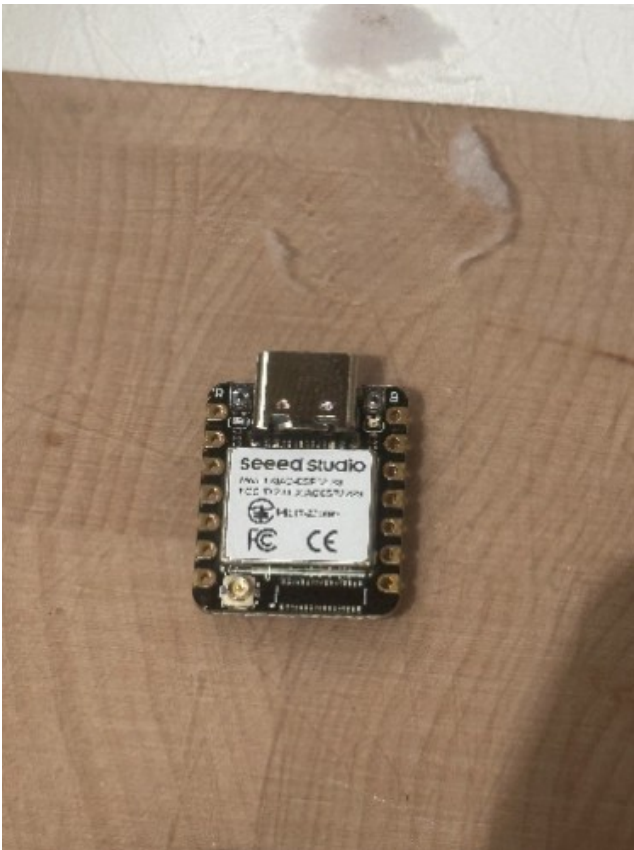
Figure 1: Seed Studio ESP32 available in the Makerspace
